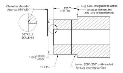
\*\*Note that .725 gives a max total of .012" bolt nose to barrel face clearance for thread an approximate .002 thread crush if barrel is to be torqued on at a value no greater than 100 ft/lbs.
